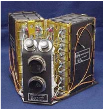
Photo of a 2 x 28 volt, 30Ah lithium ion battery designed for the Mars Rover by project team member YTP
